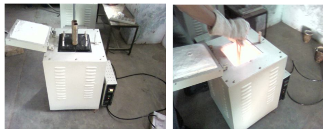
Fig. 1. (a), (b) Induction resistance furnaces with temperature regulator cum indicator.
