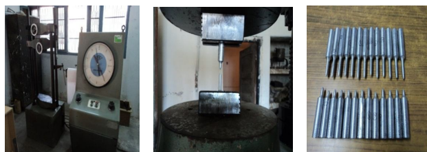
Fig. 6. (a) UTM Machine (b) Testing of specimen on UTM Machine (c) Specimens after test
