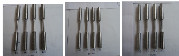
Fig. 5. Standard specimen prepared by varying the mesh size and Wt. fraction of SiC for Tensile Test
