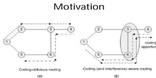
Fig. 2. Coding-oblivious versus coding-aware routing.
