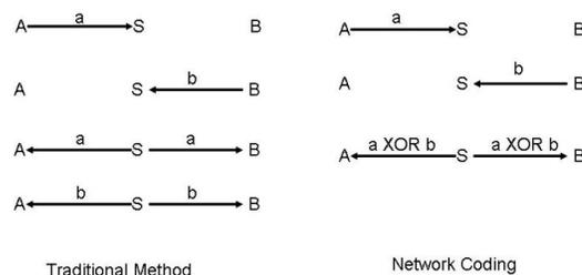
Figure.1 Network Coding versus Traditional Method of Communication.
