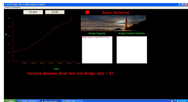
Figure 4: Ultrasonic sensor output when scour is detected
