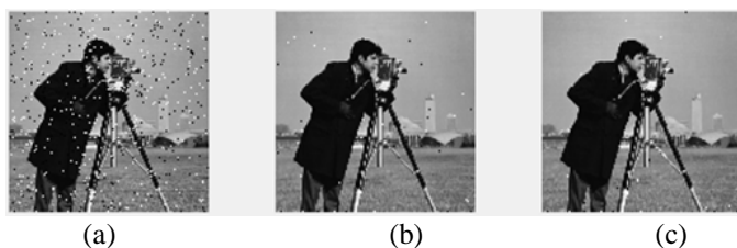
Figure 3: Comparative of Image Quality using 3X3 Mask (a) Image with 4% Noise (b) Filtered Image by Standard Median (c) Filtered Image by MF-ABV.
