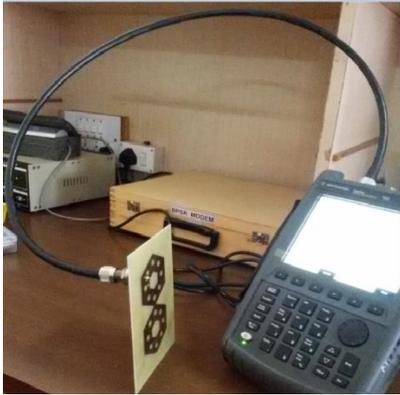
**Figure.9.** photograph of fabricated 3<sup>rd</sup> iteration
