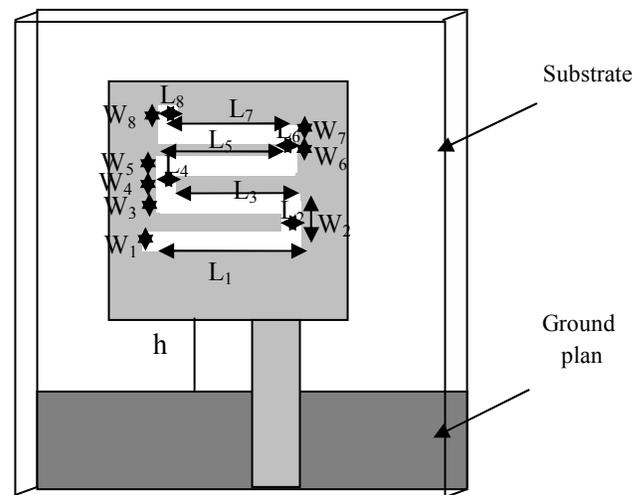
**Figure.1 :** Geometry of the antenna.
