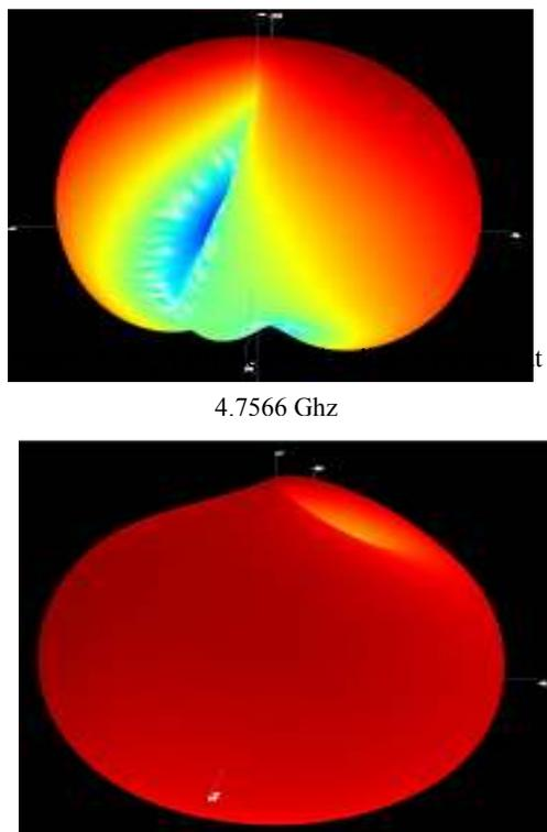
Figure 8  $E_{\phi}$  (dB) measured radiation patterns at 5.8312 Ghz
