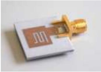
Figure. 2. UWB antenna prototype
