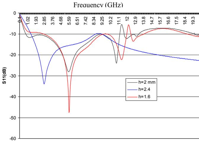
Figure. 3. Simulation returns loss the antenna for difference value of h
