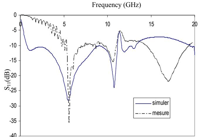
Figure.4. Measured and simulated return losses for the antenna.
