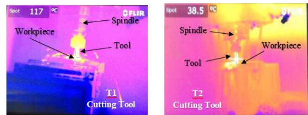
Figure 5: T1 and T2 in dry condition
