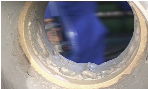
Figure 2: Wear of pump volute internal surface
