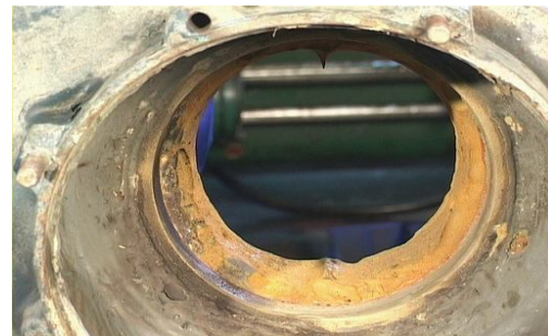
Figure 2: Wear of pump volute internal surface
