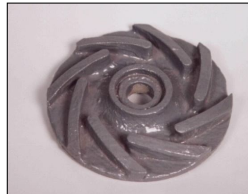
Figure 9: Reconditioning of pump impeller
