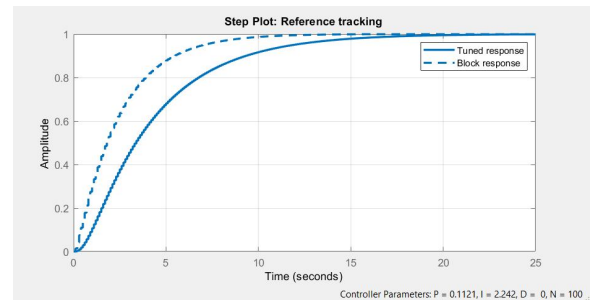
Figure 19: Current Step Response of the Controller vs. Tuned Step Response
