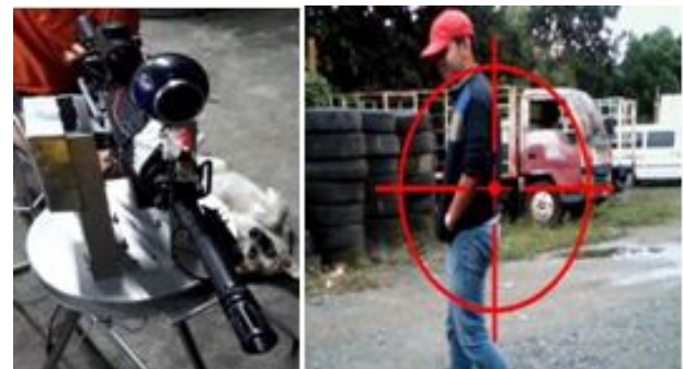
Figure 3: Airsoft Gun Web camera showing Streamed Video with Crosshair
