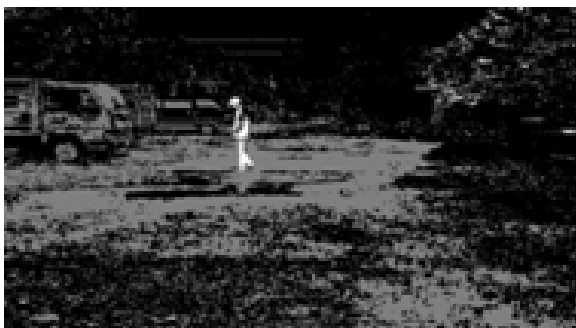
Figure 6: Output Image from the BackgroundSubtractorMOG2 function
