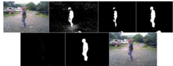
Figure 15: Morphological Operations Applied to the Video Feed
