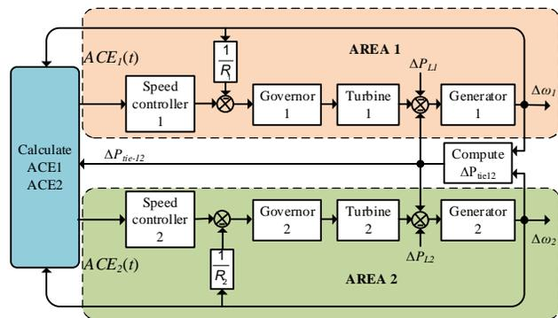
**Figure 1:** Traditional speed control strategy for a two-area interconnected hydropower system
