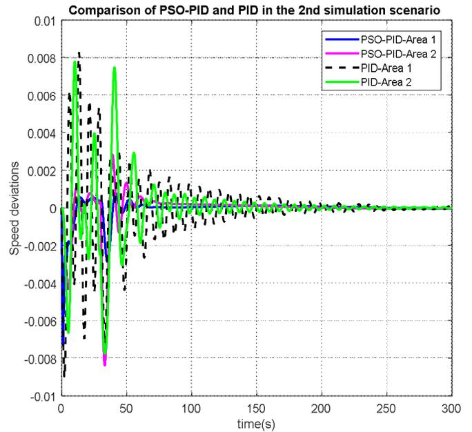
**Figure 9:** Comparison of dynamic speed deviation responses between PSO-PID and conventional PID controllers for the second scenario
