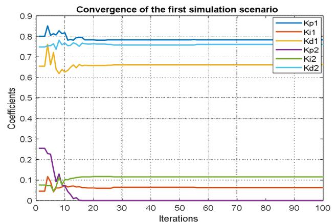
**Figure 4:** The convergence of the PSO algorithm for the first scenario
