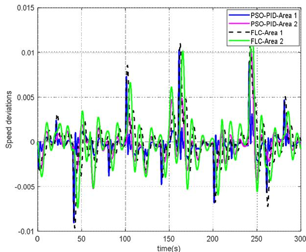
**Figure 12:** A comparison of the PSO-based PID and FLC controllers regarding the speed deviations in the third scenario
