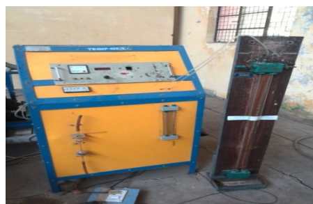
Fig. 8. Hydraulic Dynamometer with manometer
