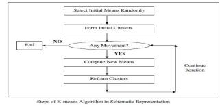
Figure 1. K-means Algorithm
