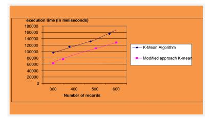
Graph shows the comparison between K-mean and Modified approach K-mean on the basis of large number of records and execution time using this algorithm. Modified approach K-mean better performance in comparison to standard K-means algorithm
