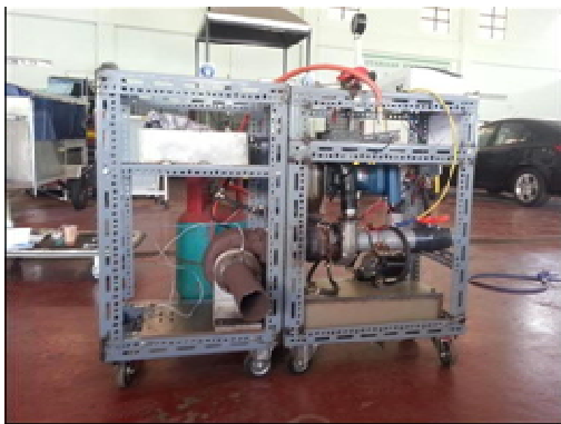
Figure 3: Developed Micro Gas Turbines
