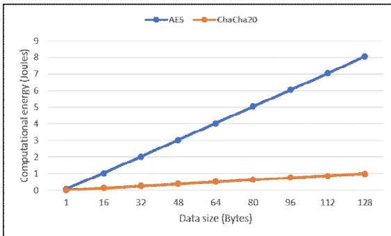
**Figure 2:** Comparison of Energy Consumption between AES and ChaCha20
