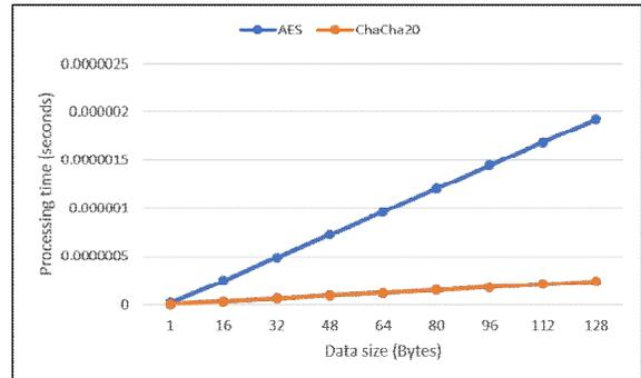
**Figure 3:** Comparison of Processing Time between AES & Chacha20
