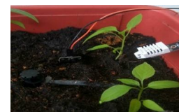
Figure 5: Moisture and DHT22 sensor location
