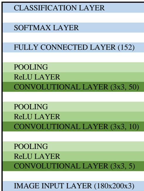
**Figure 2:** CNN Architecture of Illumination Face Recognition System
