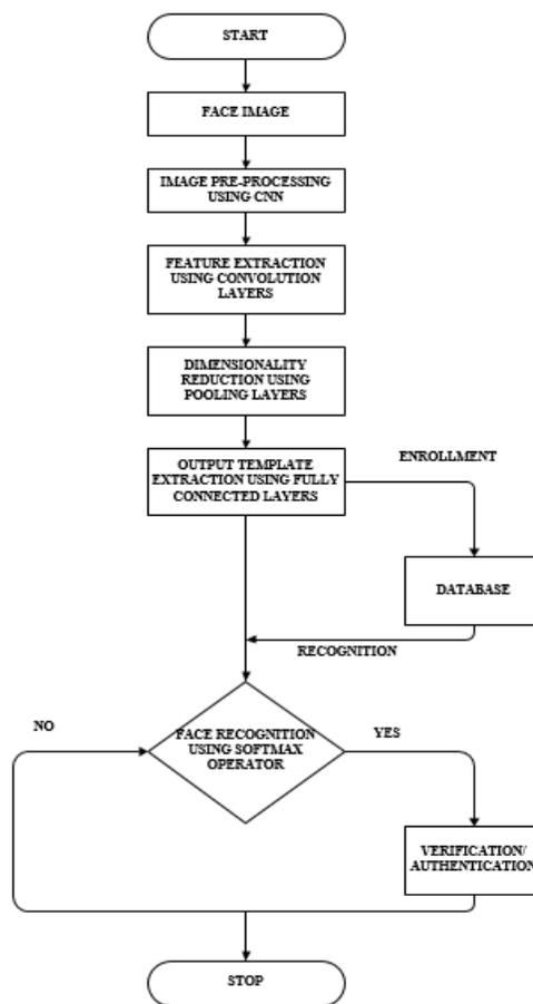
**Figure 1:** Flow chart of Illumination Face Recognition System
