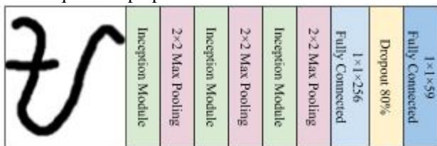
Figure 4: The complete structure of the inception network used in Baybáyin character recognition.
