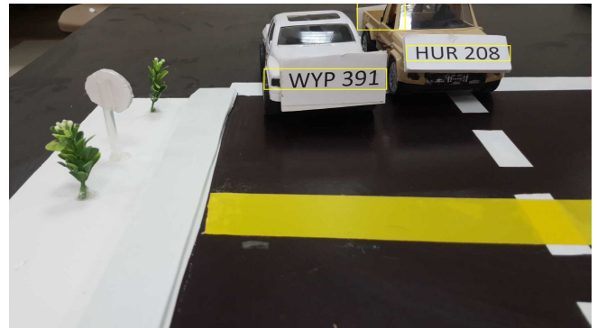
Figure 9: Recognize detected text using OCR as secondary
