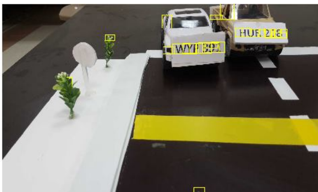
Figure 8: Merge text regions for final detection result
