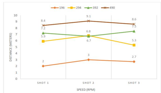
Figure 10: The distance of the shuttlecock versus the speed of the motor
