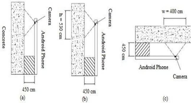
**Figure 11:** Reference image schematic capturing: (a) Distance between the camera and the concrete wall, (b) the height of the image, and (c) the width of the image.
