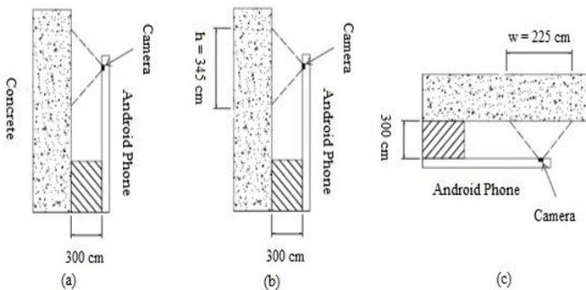
Figure 10. Source image schematic capturing: (a) Distance between the camera of an android phone and the concrete wall, (b) the height of the source image, and (c) the width of the source image.
