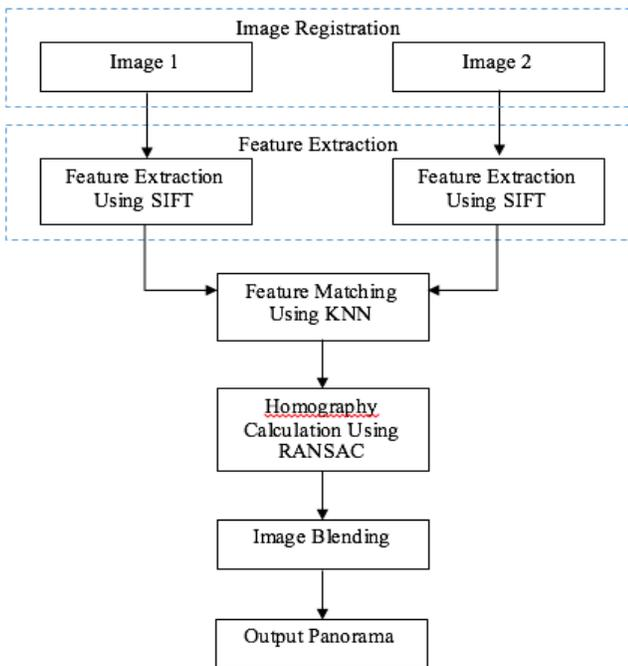
Figure 1: The block diagram of the stitching method.
