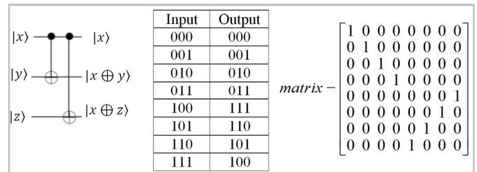
Figure 3: Type 2 modified CNOT gate.
