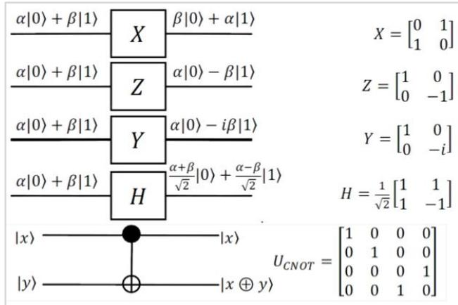
Figure 1: Basic quantum gates with matrices presentation.
