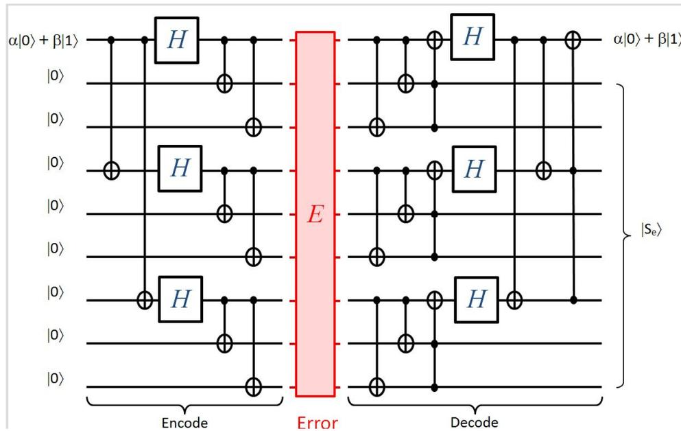
**Figure 7:**Quantum circuit for Shor code.
