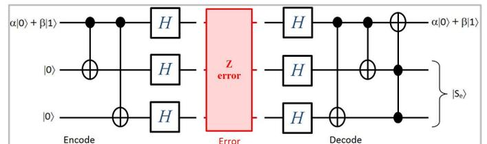
Figure 5: Quantum circuit for Z-error 3-repetition code.
