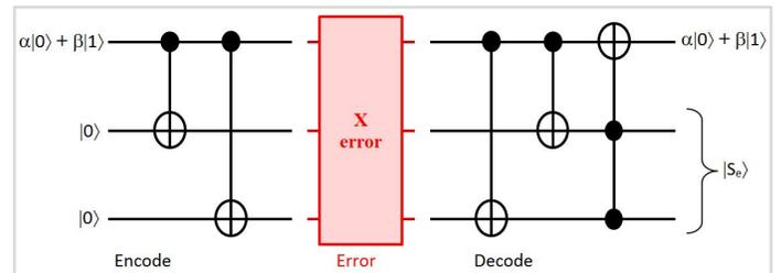
Figure 4: Quantum circuit for X-error 3-repetition code.
