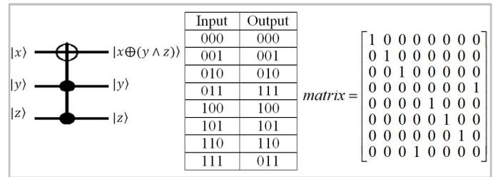
Figure 2: Type 1 modified CNOT gate.
