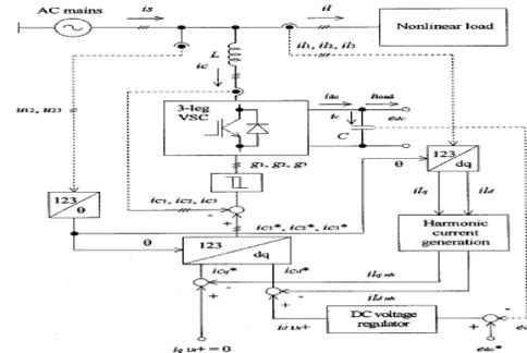
Fig.4. Control block diagram of the shunt inverter
