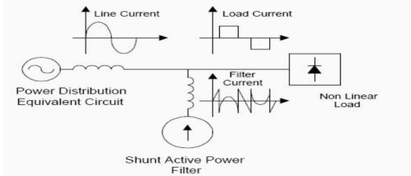
Fig 1 SAPF basic compensation principle
