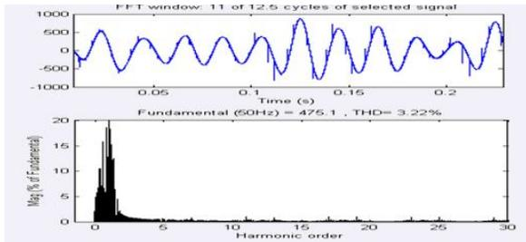
Fig19 THD Values of current waveform for dynamic diode rectifier with APF
