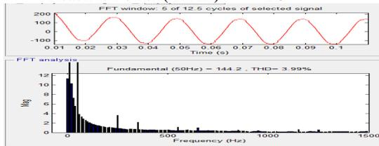
Fig12 THD Values of current waveform for diode rectifier with APF
