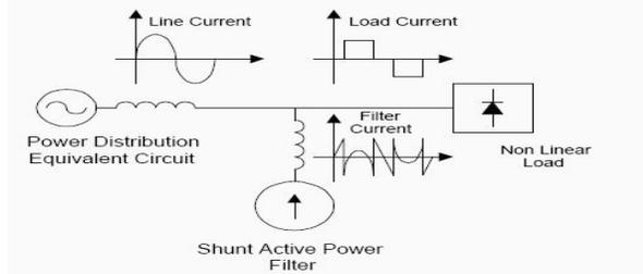
Fig 1 SAPF basic compensation principle
