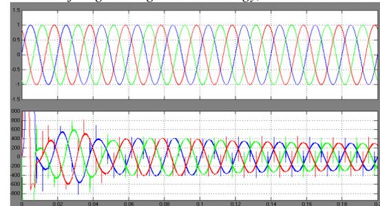
Fig15 Voltage and Current Waveforms for Thyristor converter with APF
