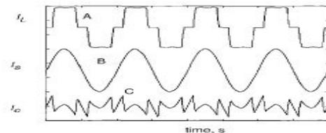
Fig 3 SAPF-shapes of (A) load, (B) source and (C) desired filter Current wave forms.
