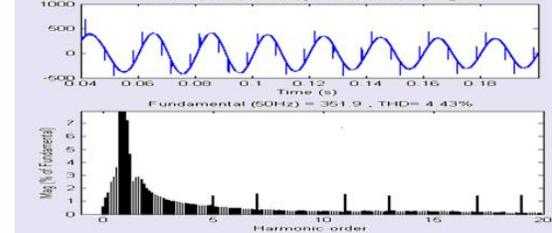
Fig16 THD Values of current waveform for Thyristor converter with APF
