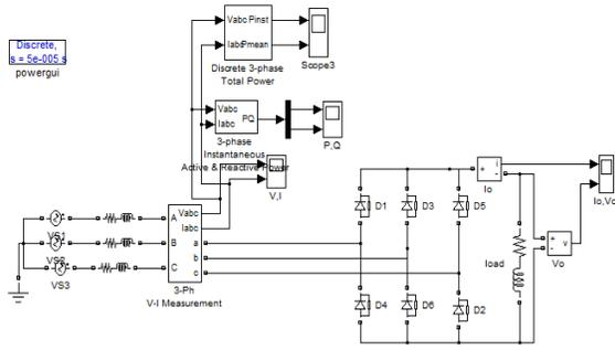
Fig 5 3-Phase source driving a diode
