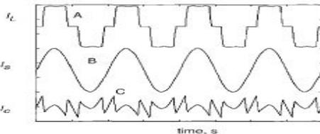
Fig 3 SAPF-shapes of (A) load, (B) source and (C) desired filter Current wave forms.
