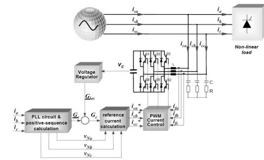
Fig 2 System configuration.
