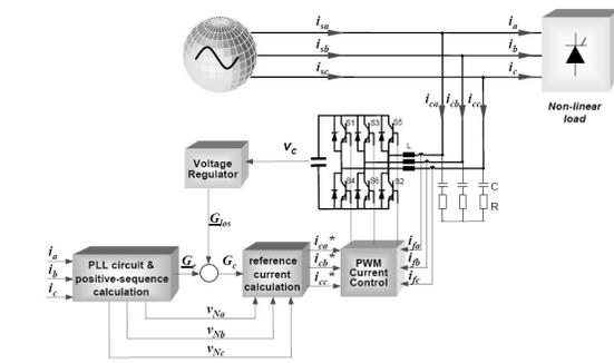
Fig 2 System configuration.
