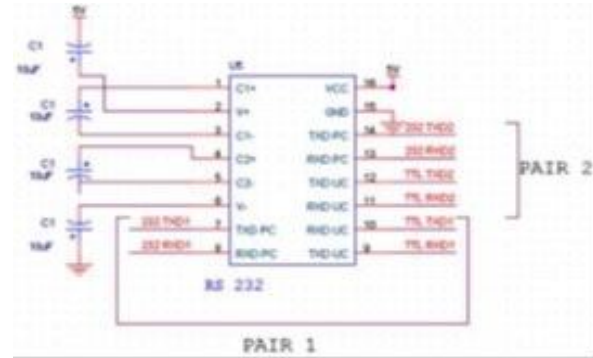
Figure.7: Interfacing of RS 232 with Microcontroller
